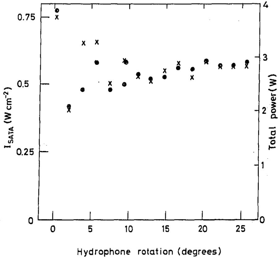
Figure 6 Variation of the results of measurements of two acoustical parameters with hydrophone rotation for a 1.5 MHz physiotherapy transducer after correcting for the directional response of the hydrophone.
