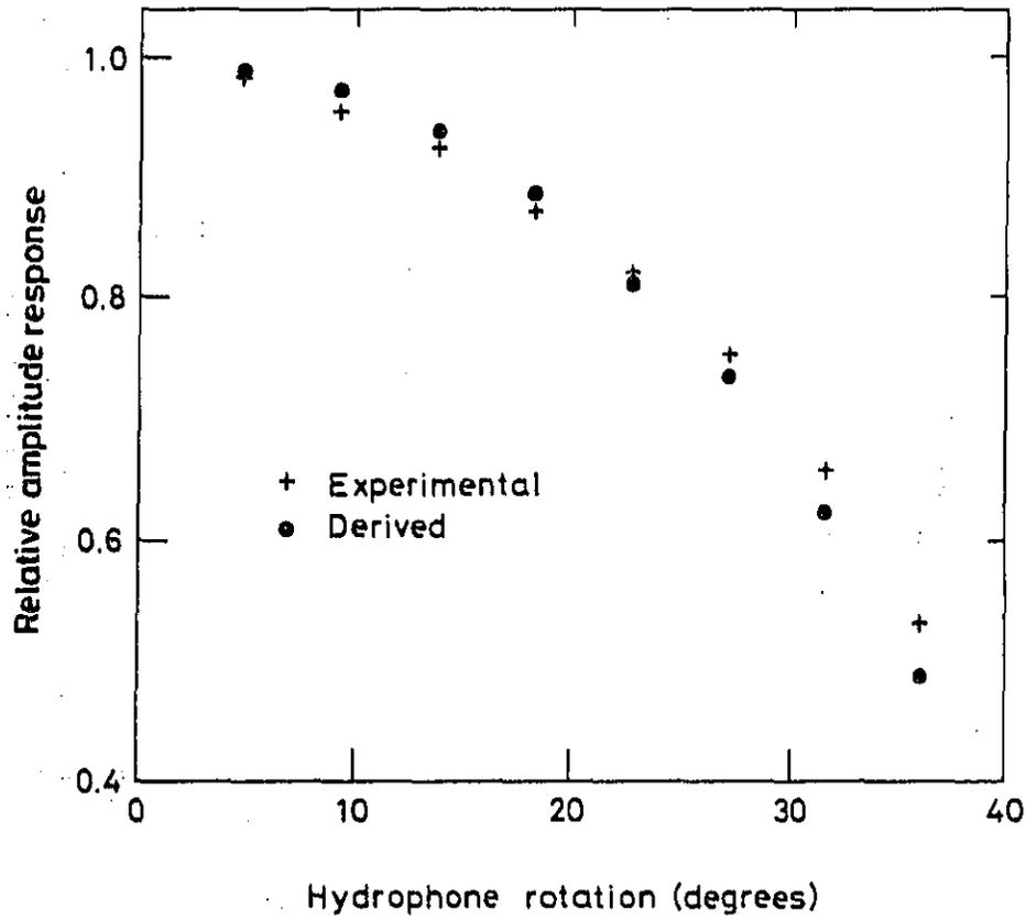
Figure 5 Comparison between the experimentally determined 1.09 MHz directional response and the 1.09 MHz response derived from the 2.25 MHz experimental data.
