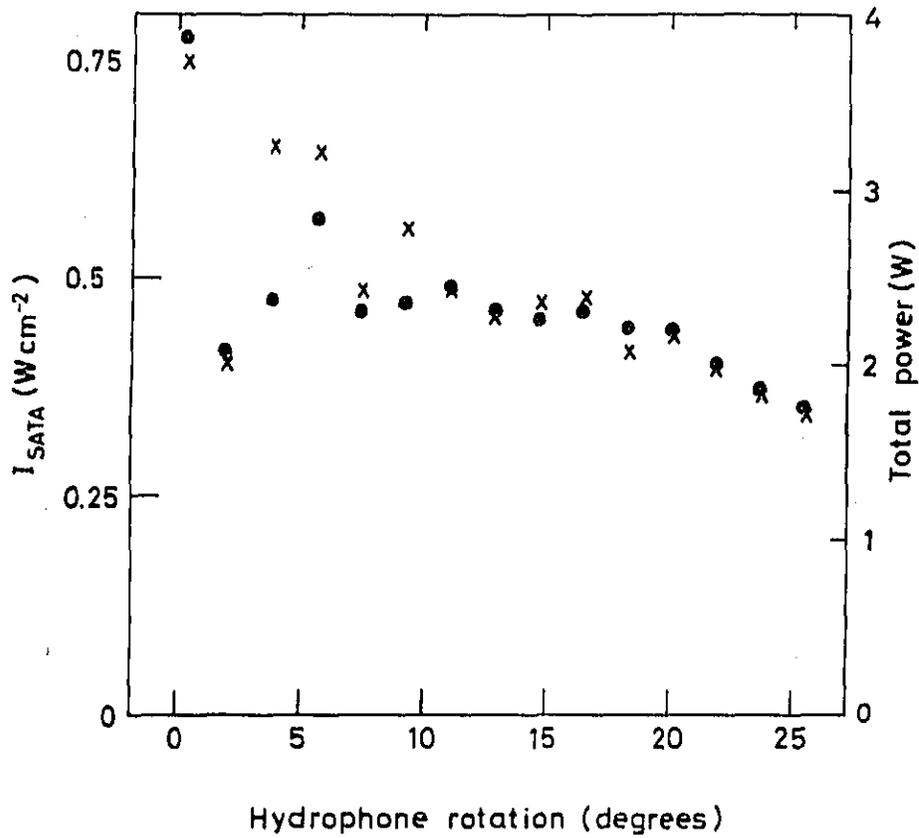
Figure 3 Variation of the results of measurements of two acoustical parameters with hydrophone rotation for a 1.5 MHz physiotherapy transducer.
