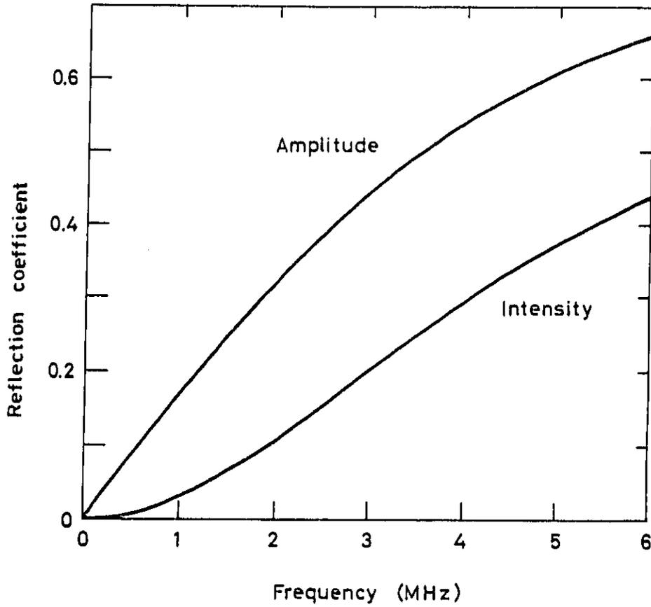
Figure 2 Amplitude and intensity reflection coefficients for a polyvinylidene fluoride membrane hydrophone of thickness 0.050 mm.
