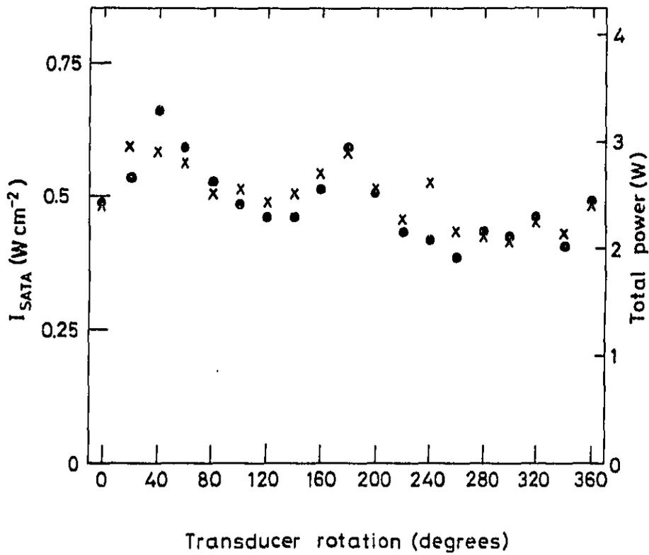
Figure 7 Variation of the results of measurements of two acoustical parameters with transducer rotation (determined at a distance of 20 mm from the face of a 20 mm diameter physiotherapy transducer operating at 1.50 MHz).
