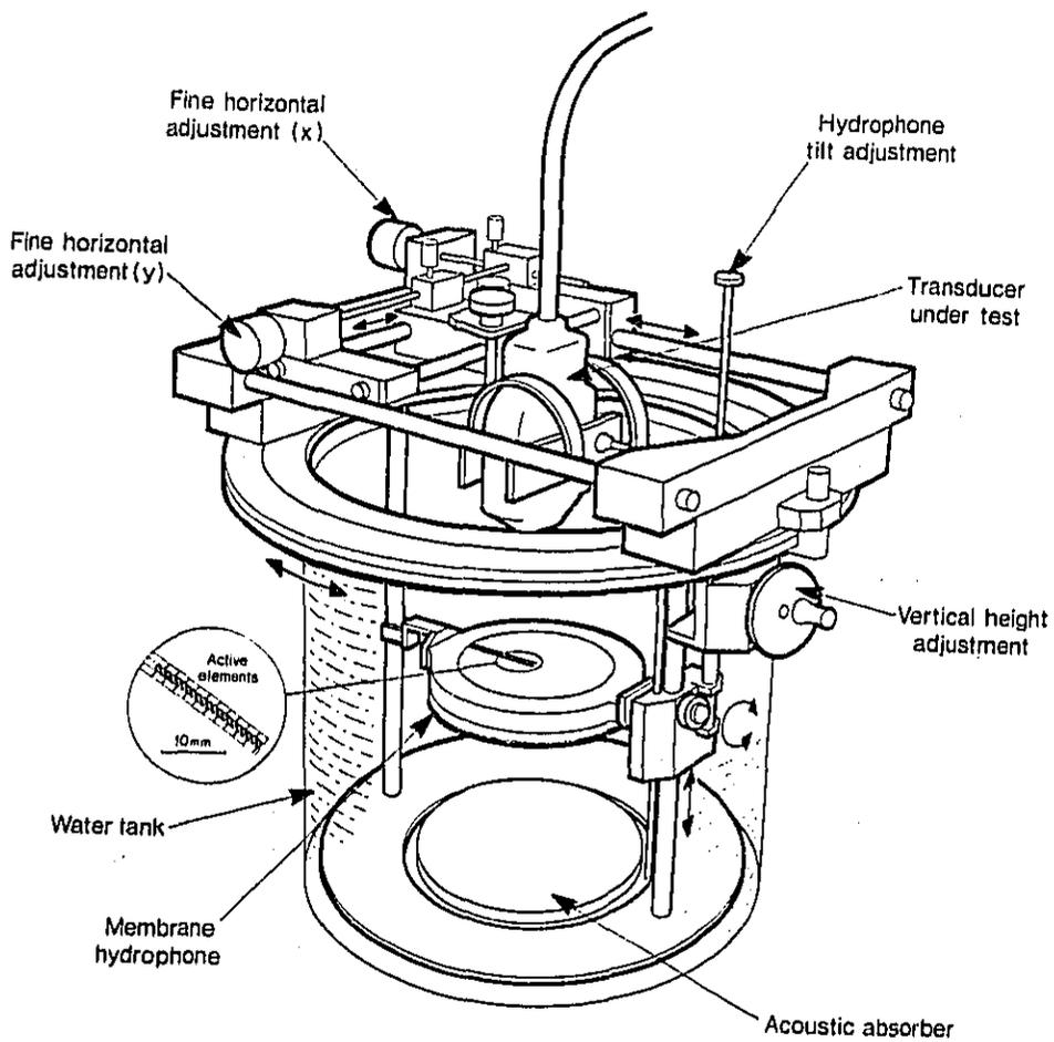
Figure 1 Schematic diagram of the test-tank used for the Ultrasound Beam Calibrator showing the various degrees of freedom available for adjusting the position of the transducer.
